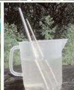
The easy to use Mechanical Bladder Pump from Geoprobe® Systems requires no expensive or cumbersome equipment. Forget about heavy generators, compressors, or pneumatic controllers, this simple to assemble pump collects representative samples of VOCs and other environmental analytes without compromising
