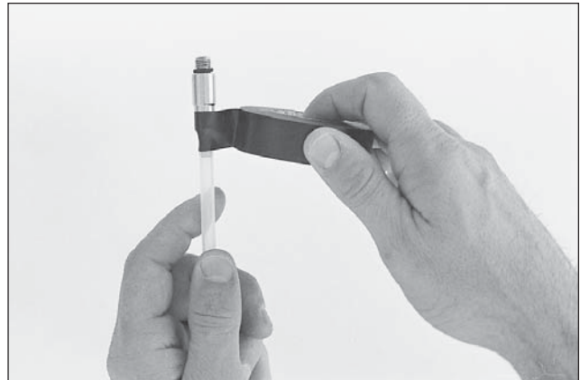
Figure 1. Securing adapter to tubing with tape. NOTE: Tape does not contact soil gas sample.
