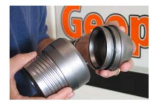
eliminate problems when sampling in saturated sands. This also prevents the Expendable Cutting Shoe from being unintentionally released from the Expendable Cutting Shoe holder.
